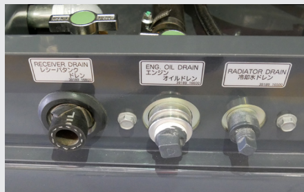
Easy to service - External fluid drain points
